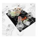
Acrylic (PMMA) is a transparent, electrically insulating thermoplastic offering good stiffness, excellent optical clarity, and resistance to many aqueous chemicals and detergents. It is not resistant to many organic solvents and should be used within the stated service temperatures.
