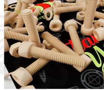
Polyether ether ketone (PEEK) is a high-performance, semi-crystalline engineering plastic known for its exceptional properties. It offers robust chemical resistance, with concentrated sulfuric acid being the only common chemical capable of dissolving it. PEEK also boasts outstanding heat resistance, wear resistance, flame retardancy, and hydrolysis resistance, making it ideal for demanding applications.
