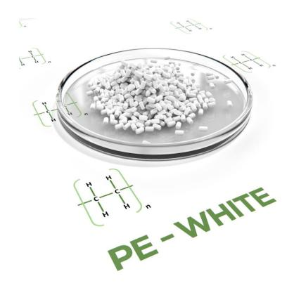
Lightweight polyolefin with good chemical resistance and electrical insulation; moderate stiffness and low friction.
