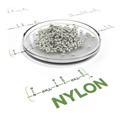
Strong, tough polyamide with low friction and excellent wear resistance; moisture-sensitive with property shifts when conditioned.
